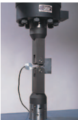
Grips for CT specimens with clip gauge
