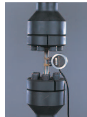
Dynastrain (measures displacement between gauge marks)
