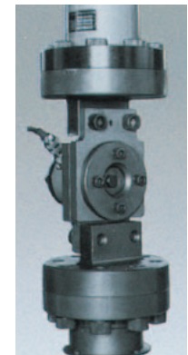
Thread-loosening test jig
