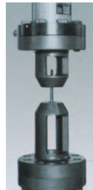
Tensile test jig for fatigue testing of bolts
