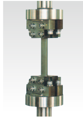
Manual non-shift grips for flat specimens
