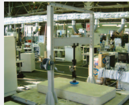
Customized system example: bed durability evaluation system
